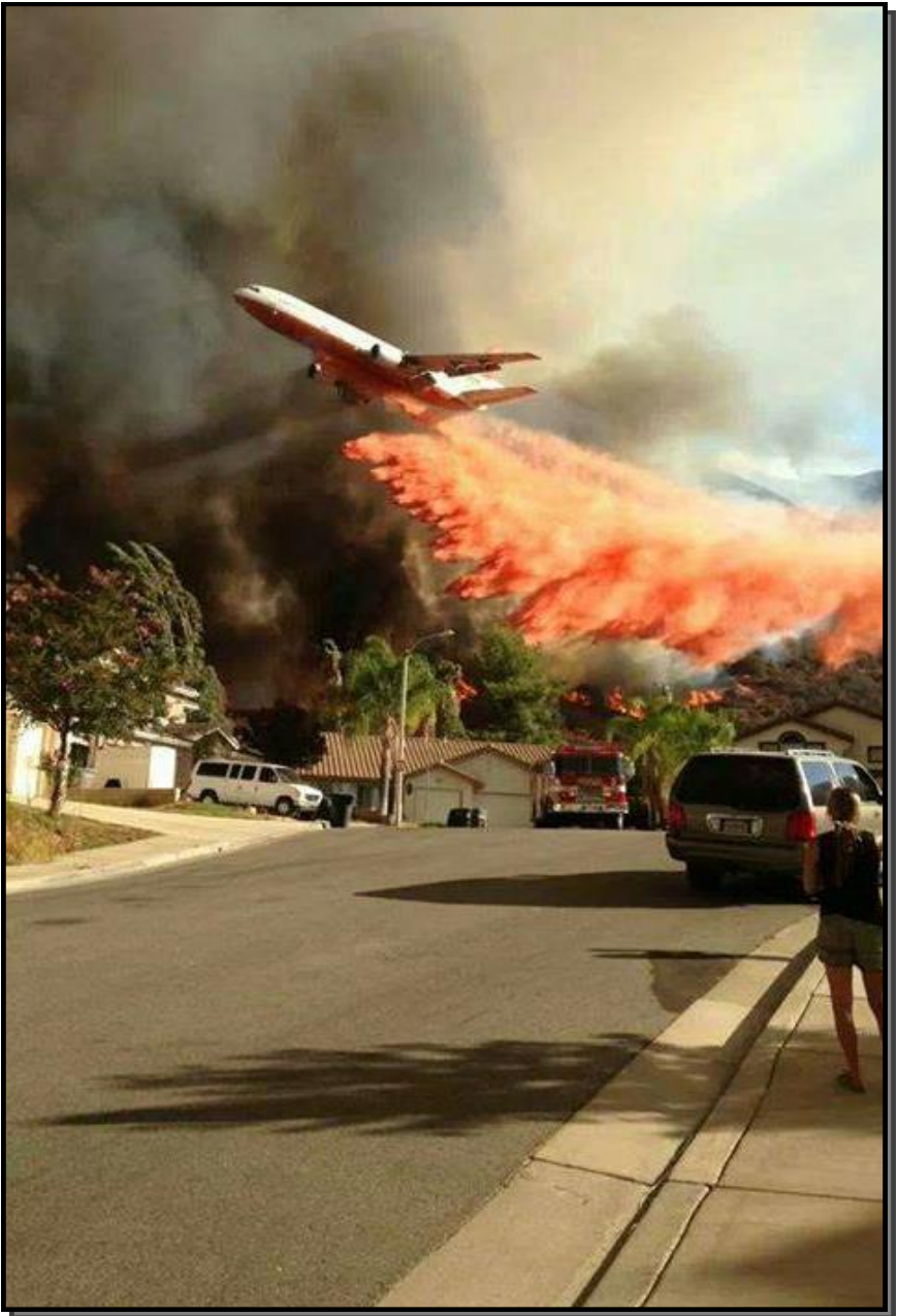
The DC10 VLAT making a timely retardant drop on a brush fire in the Lake Elsinore area of Riverside County. Photographer unknown
